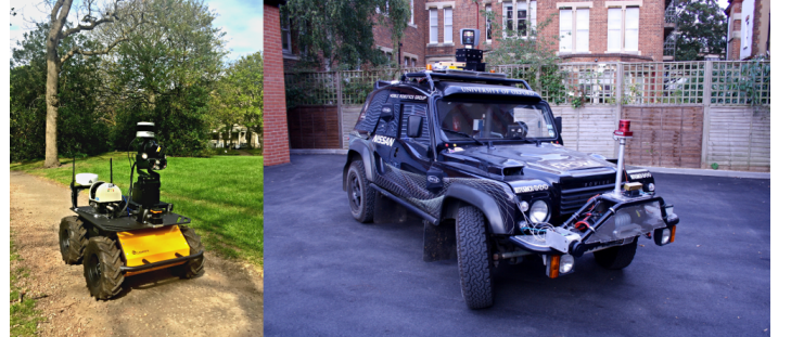
Fig. 5: The robots utilized to collect data for our experiments. A Clearpath Husky robot (left) was used to collect the GS dataset with a push-broom LIDAR and a Multisense SL. A Bowler Wildcat platform (right) was utilized to collect the CP dataset, equipped with a Velodyne HDL-32E LIDAR, Oxts GPS, Novatel INS and Bumblebee 2 camera.
