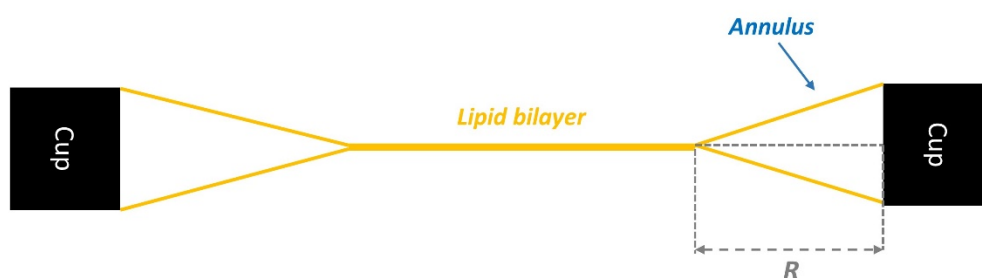
Figure 2.5 Forces involved in the formation of a planar lipid bilayer
