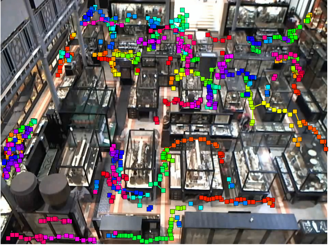
Figure 3.4: Tracklet generation: The figure shows the tracklets that have been generated by the proposed technique over a period of 120 frames. The squares indicate camera detections. Squares of the same colour indicate that these detections originate from one target with high confidence and so are linked together.
