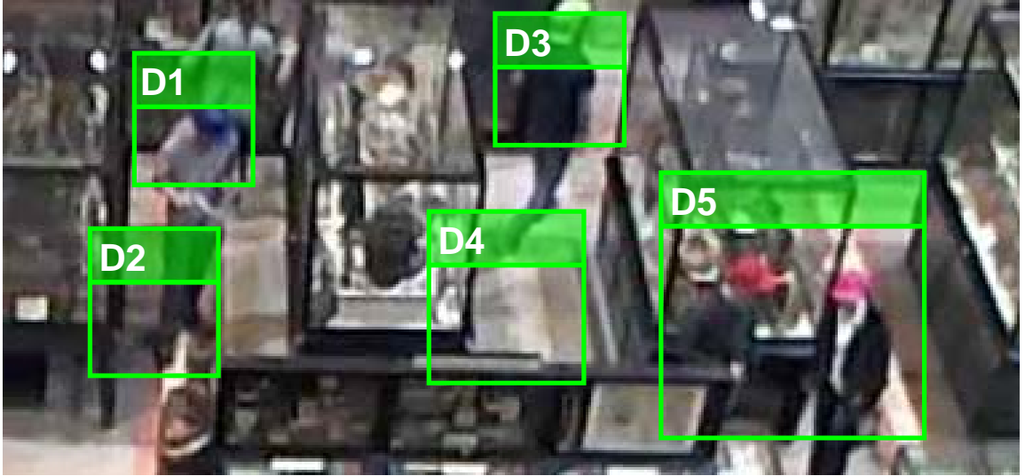
Figure 3.3: Three cases of noisy detections generated by our visual-based detector: a) multiple detections are generated for one moving target (D1 and D2), b) a detection contains no moving targets at all (D4), and c) one detection contains multiple moving targets (D5).
