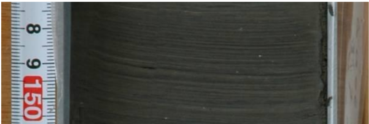
Figure 3.6: Magnified view of a section of the Lake Suigetsu sediment core from the present study (SG06 core section B-18, composite core depth 3593.1 to 3596.7 cm), demonstrating the clear laminations present throughout the sediment profile.
