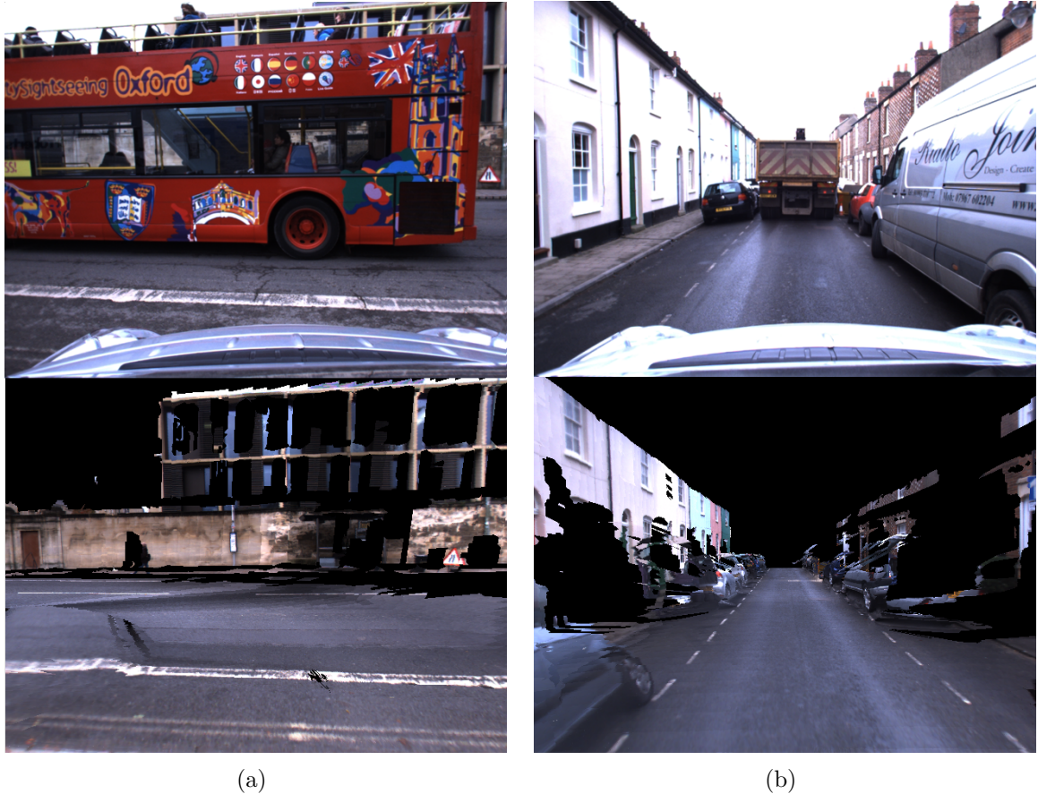
Figure 4.18: Localisation failures due to dynamic obstacles. Top: camera image, Bottom: map. Too little of the static scene is visible for the camera images to be matched against the map.
