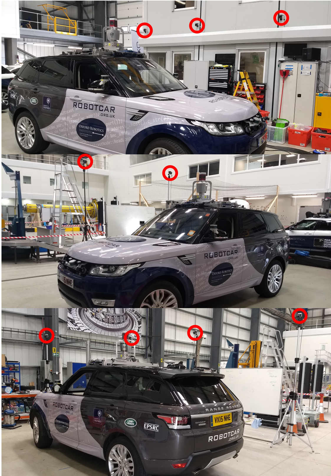
Figure 5.8: Vicon setup used for validating calibration. The Vicon cameras are circled in red.
