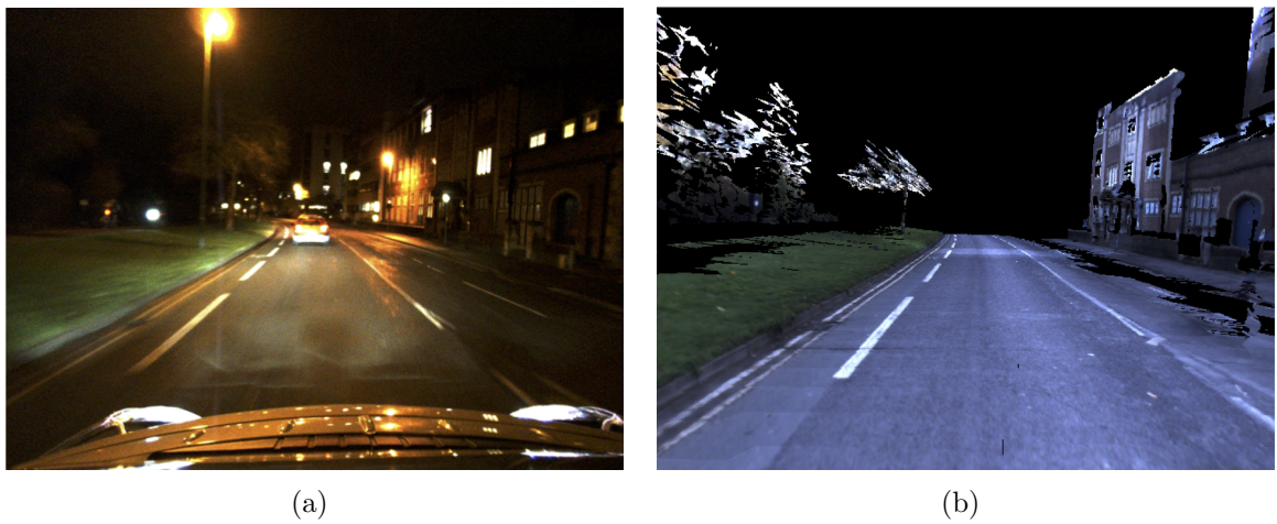
Figure 4.19: Example of a night-time image for which localisation fails. Left: camera image, Right: map. The light distribution in the scene is very different to that during the day, partially due to a light source that moves with the vehicle.
