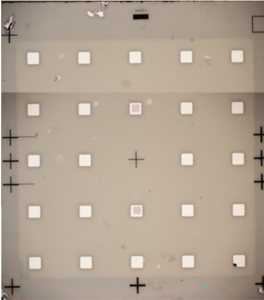
FIGURE 7.8: The boron-doped diamond sample after full process and ready-for-testing. patterned aluminium Schottky contacts visible above each laser-written array of columns.
