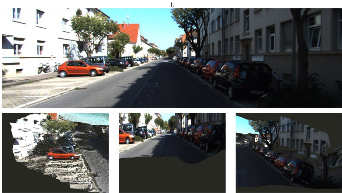
Figure 5.5: An example scene showcasing depth map estimation of an urban scene. From the reference image (top) it can be seen that the variational technique struggles with the large, plain and planar surfaces with the walls (bottom left, bottom right) being estimated noisily while an erroneous estimate is made for the similarly plain road (bottom middle).
