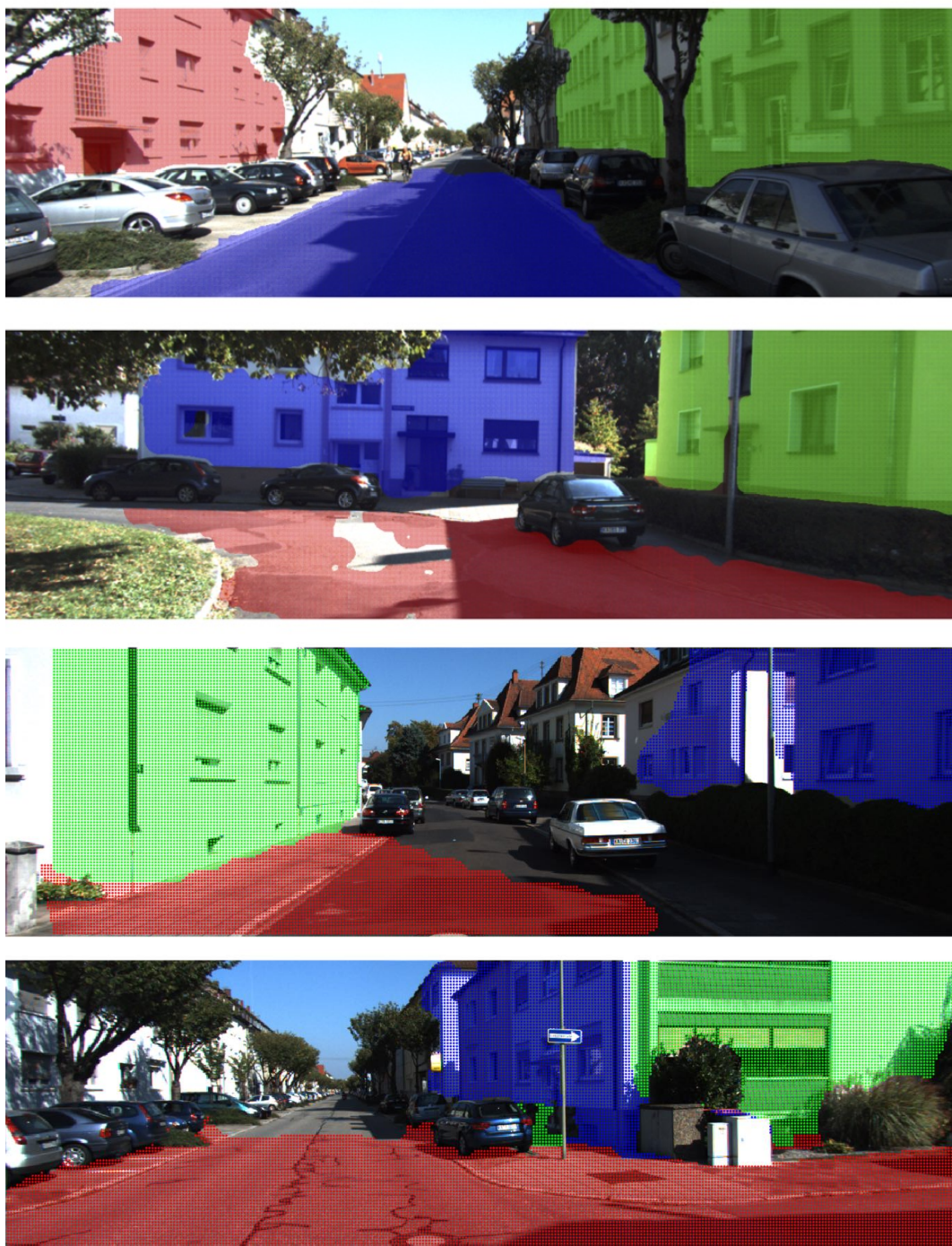
Figure 5.10: Sample results showing planar prior pixel labelling through an energy minimisation approach. This leverages planes obtained through CORAL and assigned pixels to them through a planar prior labelling. From planar priors obtained using CORAL pixels are assigned to these priors using a global energy function. The depth of these pixels can then be estimated solely using the plane hypotheses.
