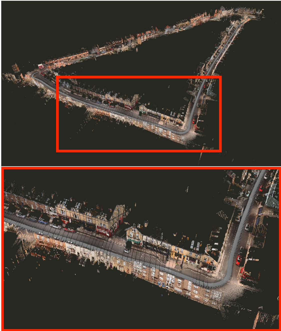
Figure 7.1: A large scale reconstruction obtained as solution of the graph optimisation, proposed in this chapter, over a 2km trajectory of an urban environment (top). By combining two different sensor modalities, a push broom laser and a stereo camera with a known cross-calibration, we can create low-cost reconstructions of the environment, these are however subject to "drift" that impacts their accuracy. In this chapter we offer a unified framework to handle multiple architectural constraints driven by the different geometric features discovered in the environment (e.g. points, planes, etc), these constraints can then be employed to improve the motion estimation resulting in accurate reconstructions over large-scales (bottom).
