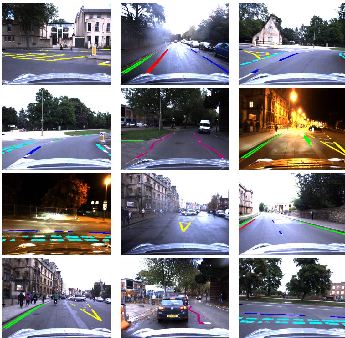
Figure 6.7: Sample of results from the semantic classification of road marking pixels under different weather and lighting conditions (overcast/rain/night). Our proposed CORAL approach is able to detect multiple road marking segments in images from detected road marking pixels. These segments are aggregated through another energy minimisation into their semantic classes. Thereby we reveal the underlying meaning of the road markings in complex urban environments providing important cues for autonomous vehicles. These include indicating for upcoming road situations, which could require specific behaviour. For instance, the zig-zag markers ( purple ) indicate an upcoming pedestrian crossing and the give-way dashes ( cyan ) indicate a junction.
