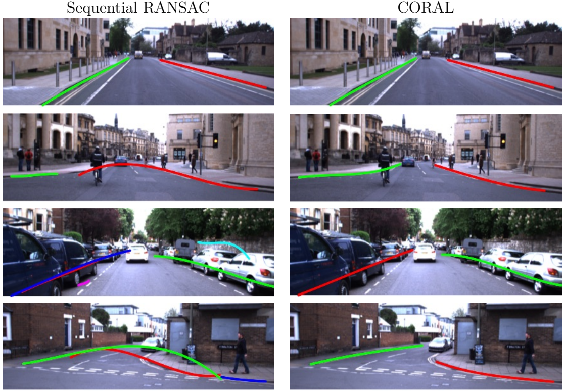
Figure 6.13: Comparison of results of geometric road boundary fitting from the output of the combined networks using Sequential RANSAC and CORAL. While CORAL is able to obtain the minimum set of cubic curves that represent the road boundaries, without any prior information of the number of models, in a diversity of viewed scenes the performance of RANSAC deteriorates in the presence of noise and in more complex scenes returning inaccurate road boundary models.
