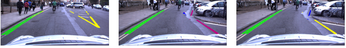
Figure 6.8: Given a fully observed road marking (left) our proposed approach is able to correctly detect the underlying semantic class of the road markings on a image. However when this becomes partially observed (middle) the interaction of the underlying geometric primitives with others in the scene can cause mis-classification, in this case the road junction was labelled as a zig-zag line. By introducing road marking tracking (right) even under partial observation the correct underlying can be arrived at, making the classifications more robust.
