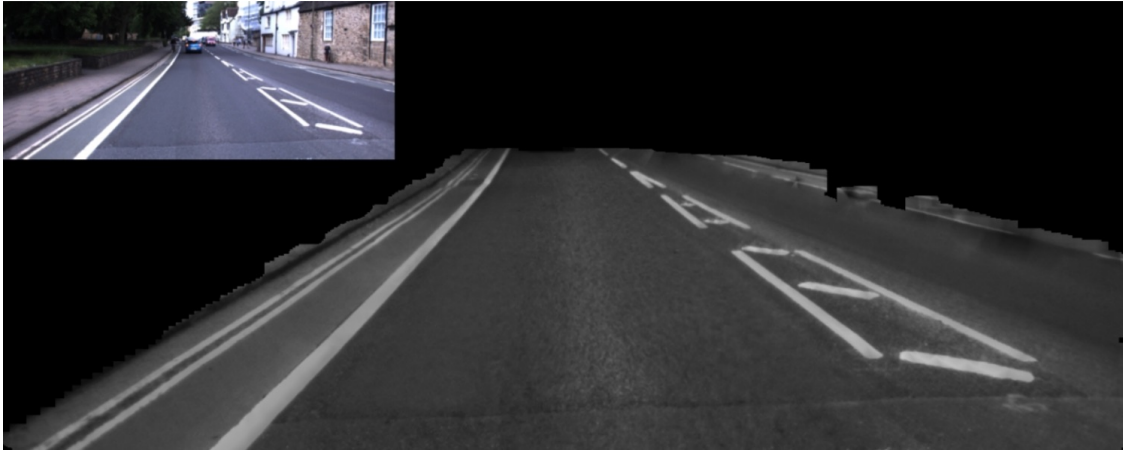
Figure 6.2: Figure showing a LiDAR point cloud of a road surface and the corresponding camera image of the same scene. It can be seen that the high-reflectance pixels correspond to road markings which can be related to the image pixels using a Conditional Random Field.
