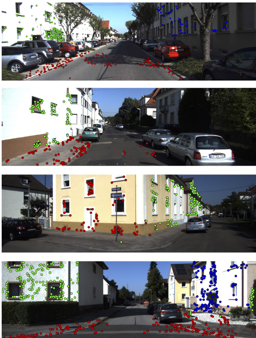
Figure 5.8: Sample of the results from multi-homography fitting using CORAL with membership to different homographies encoded by colour-coded. CORAL can be seen to capture the large, plain and planar surfaces through the homography models in a variety of scenes and plane orientations. The planar priors can then be obtained through homography decomposition.
