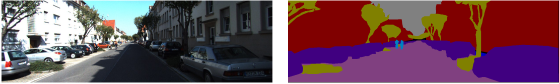
Figure 5.9: Semantic Segmentation of the pixels of an image (left) into its respective classes (right). Buildings and roads over which planar surfaces are expected to be found are labelled in red and pink respectively.
