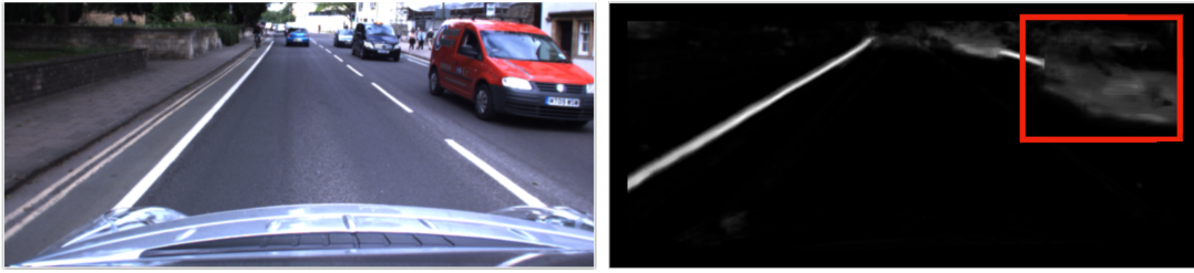
Figure 6.9: Given an input image (left), an adequately trained deep segmentation network is able to correctly identify the visible road marking pixels. However it produces a blurry output through occlusions (red rectangle) as it is unable to infer the underlying geometry that persists through the occlusions which would bias it to correctly detect the occluded road boundaries.
