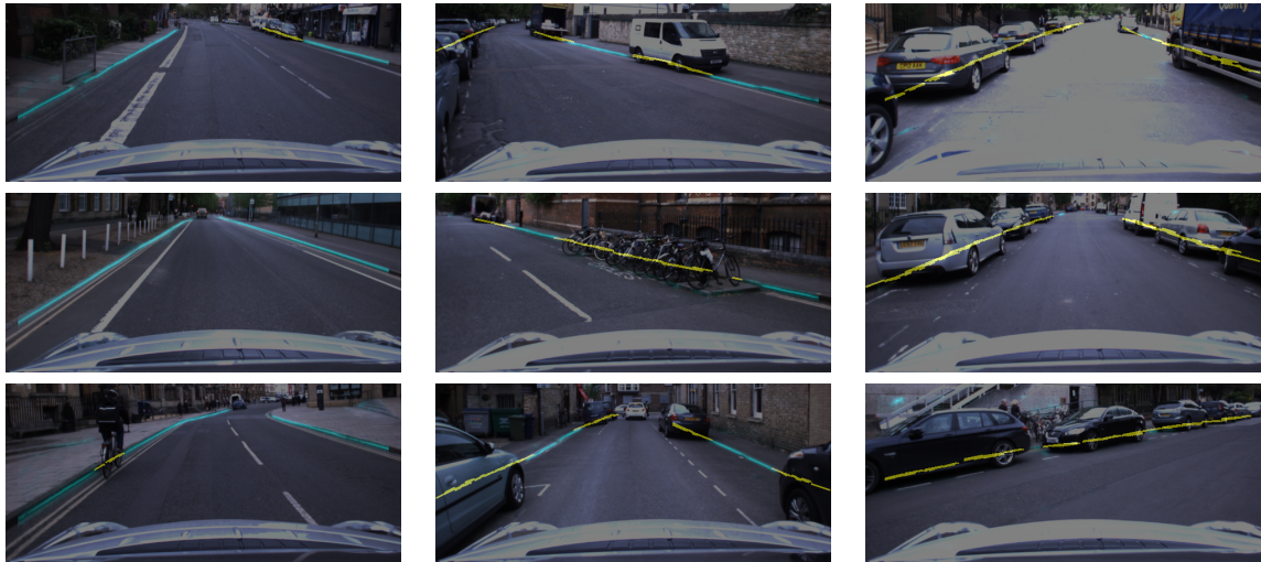
Figure 6.12: Sample outputs from the combined networks under different levels of road boundary occlusion. These are able to seamlessly deal with and predict the position of the road boundaries in scenarios of low to no occlusion (left), some occlusion (middle) and full occlusion (right). The blue pixels are the visible road boundaries while the yellow pixels represent the occluded boundaries.
