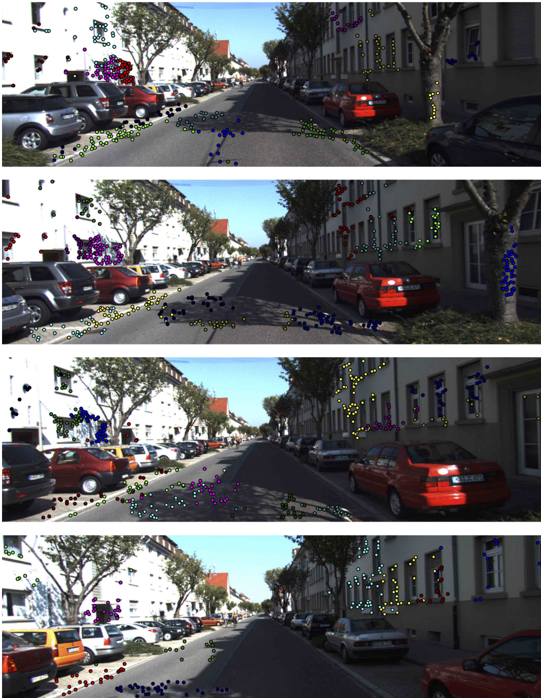
Figure 5.7: Figure showing multiple homography initialisation using affine transformations and affinity propagation clustering. With membership to a specific homography coded by colour it can be seen that this method results in an over-segmentation with a prevalence of redundant models.
