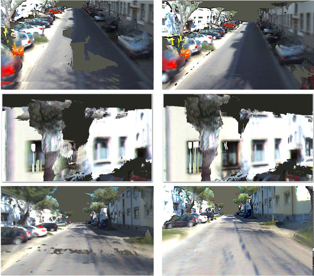
Figure 5.13: Sample results of dense reconstructions from the fusion of depth maps in the two evaluated sections are shown in this figure. The left column of images corresponds to the reconstructions produced using the TGV depth maps. It can be seen that the noise on the depth maps results in some gaps in the reconstruction. By improving these depth maps with planar priors in our approach the results can be improved on, significantly, as shown in the right column. Resulting in a more accurate map of the world.
