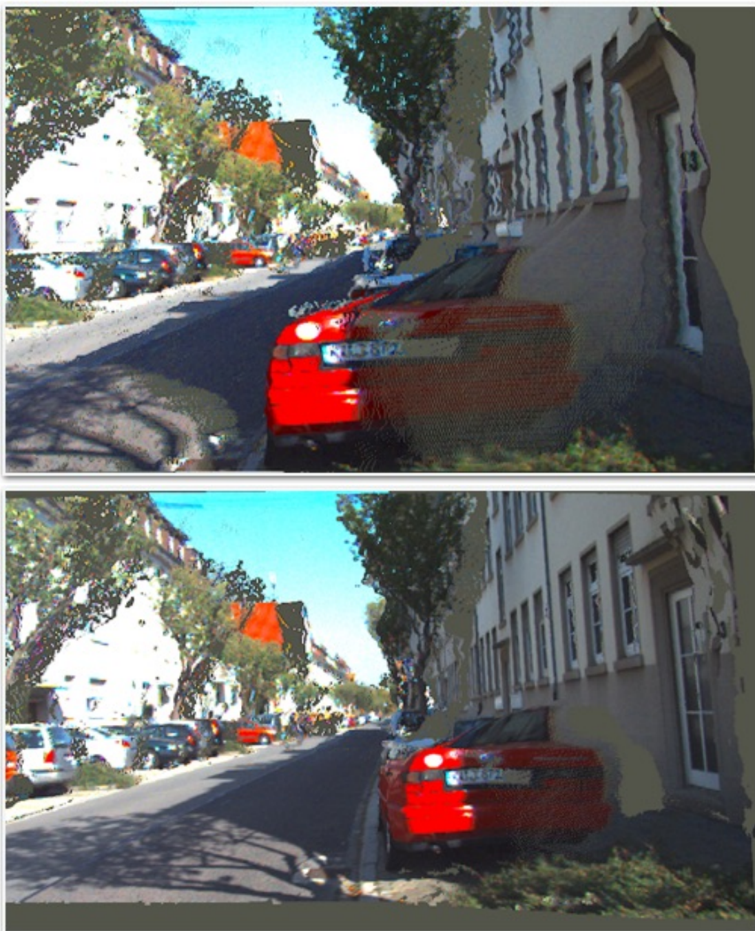
Figure 5.2: A qualitative perspective of this chapter. A dense depth map projection (top) of a planar wall surface created by a state-of-the-art Total Generalised Variation algorithm is displayed. As expected, the algorithm results in a noisy output on the largely textureless wall and road. CORAL discovers planar regions and from there invokes a planar prior to restricted areas. This results in an improved depth map projection (bottom), showing a marked improvement in the depth estimation along the wall and road.
