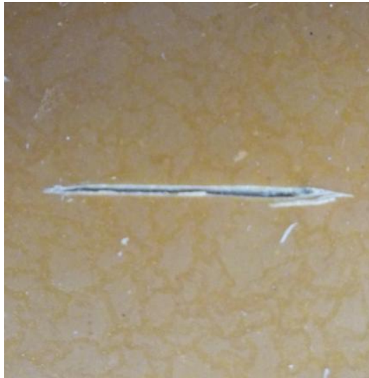
Figure 6.26 – Digital photograph of defected \text{Ce(dpp)}_3 Epigen coating immersed in 2M NaCl for 7 days
