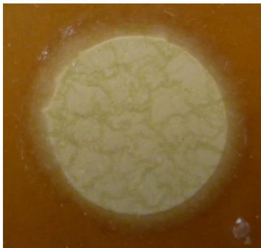
Figure 6.22 – Digital photograph of fully intact \text{Ce(dpp)}_3 Epigen surface immersed in 2M NaCl
