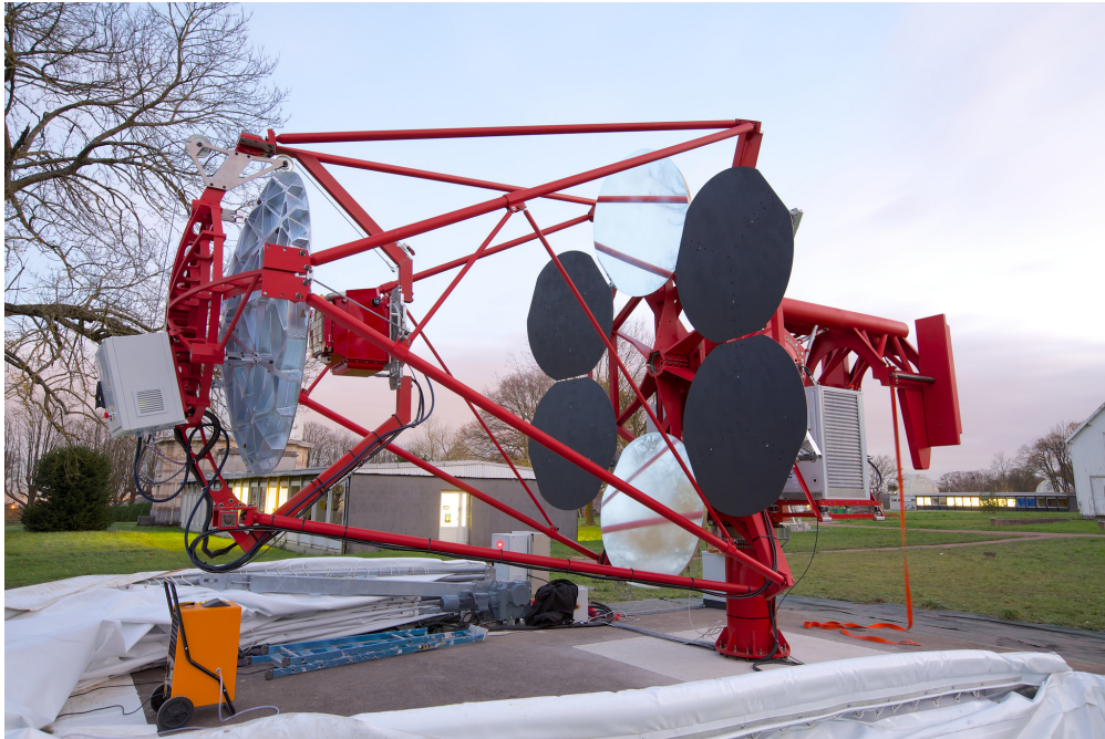
Fig. 1.22 Picture of the prototype telescope structure at the Observatoire de Paris in Meudon, France. Four black machined dummies substitute the, at that time, missing mirrors.
