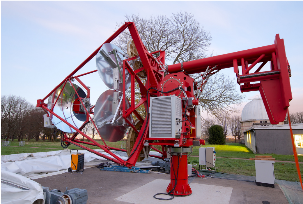
Fig. 5.3 Chiller mounted at the side of the telescope structure.
