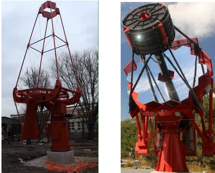
Fig. 1.20 Picture of the SST-1M prototype structure (left; without mirror) and of the ASTRI telescope (right). Credit to the respective collaborations.
