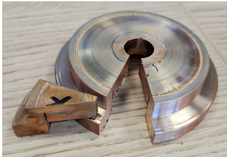
Figure 5.7: Electron-beam weld on a test piece for the upper endcap. The location of the weld can be seen by the burred edge. Notably, there are no signs of the weld in the cross-section.
