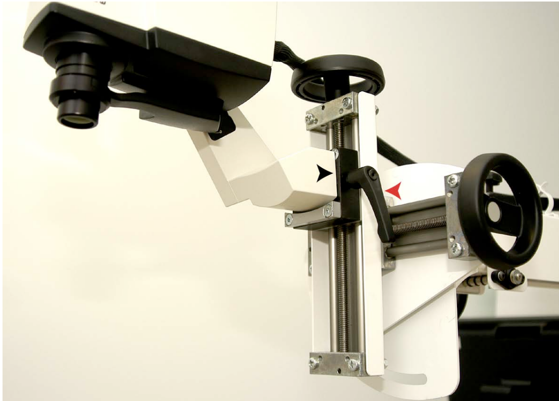
Figure 1.47: Multi-positional bracket of the modified Heidelberg Spectralis imaging system
