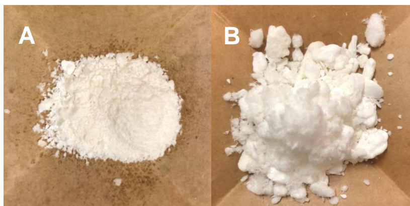
Acid grade fluorspar derived Me 4 NF· t AmOH (A) and Bu 4 NF·( n BuOH) 4 (B)
