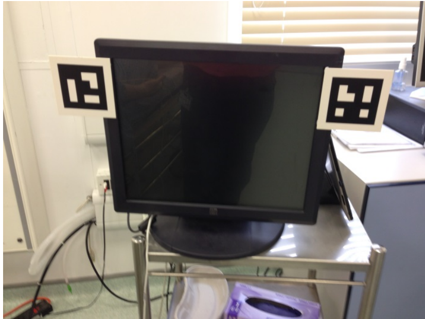
Figure 10-1: Image of a patient monitor configured for the simulation experiment described in chapter 8. Note the 'Region of Interest' markers affixed to either side of the screen to enable the system to track target regions.
