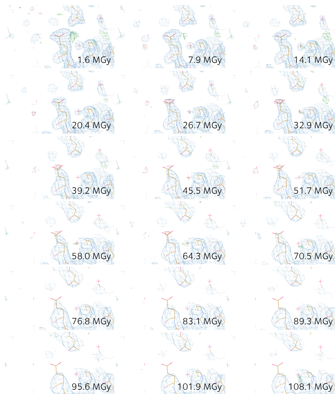
Figure 4.14: Electron density maps (blue) of the GLU 155 residue in the DY2A4 radiation damage series plotted at 1.0\sigma level. F_{\text{obs}} - F_{\text{calc}} difference electron density (red negative, green positive difference) plotted at 3.0\sigma .
