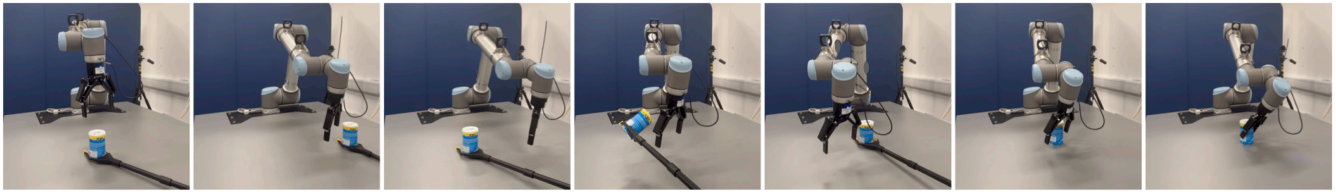
Fig. 10: Grasp-MPC execution for moving objects. Grasp-MPC adapts in real time to track and grasp moving target objects, capabilities that open-loop approaches lack.
