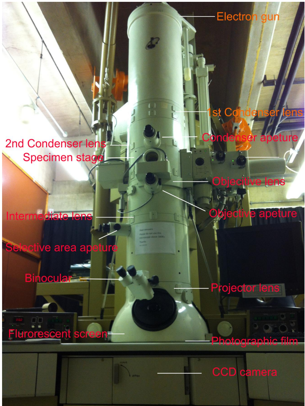
Figure 2.1. The structure of JEOL 4000 HRTEM used in this thesis, located in department of materials, University of Oxford.
