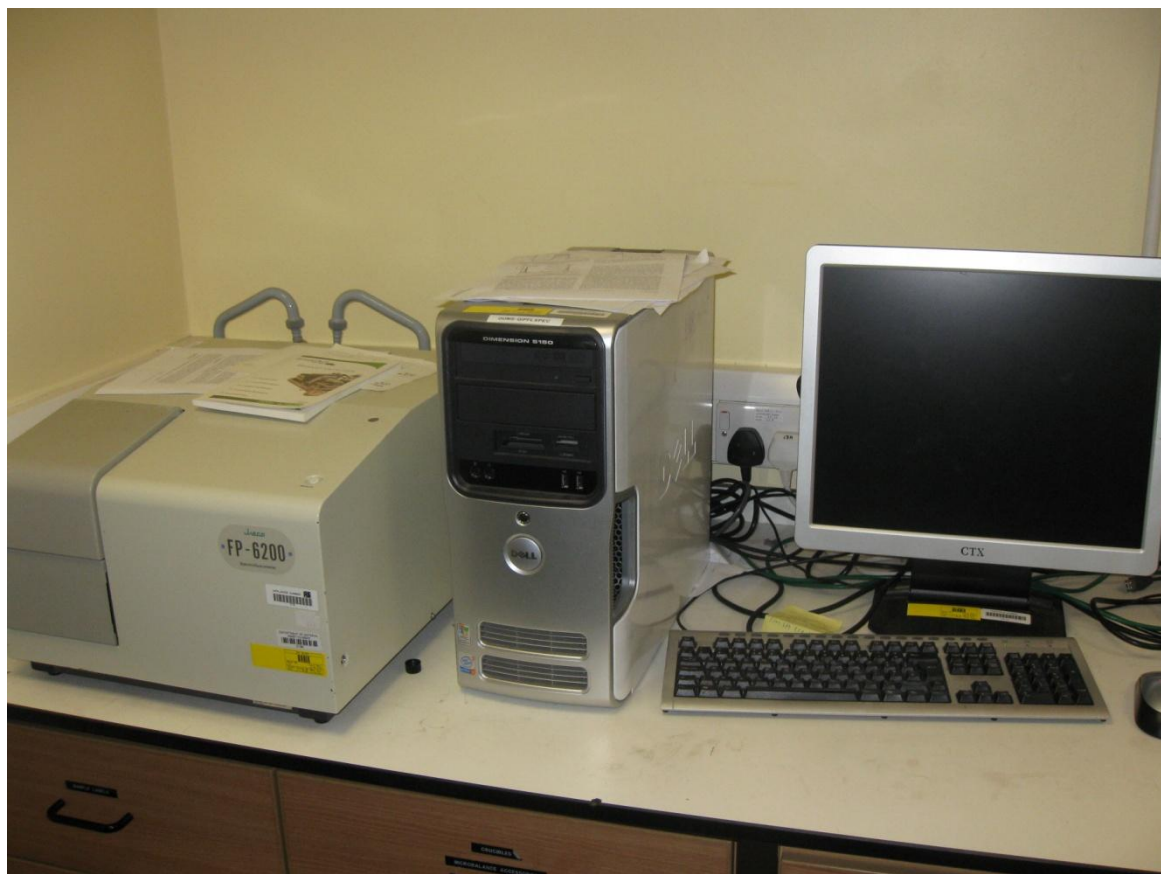
Figure 2.18. JASCO FP-6200 PL/PLE spectrometer used in this thesis, located in 12/13 parks road, department of materials, University of Oxford.
