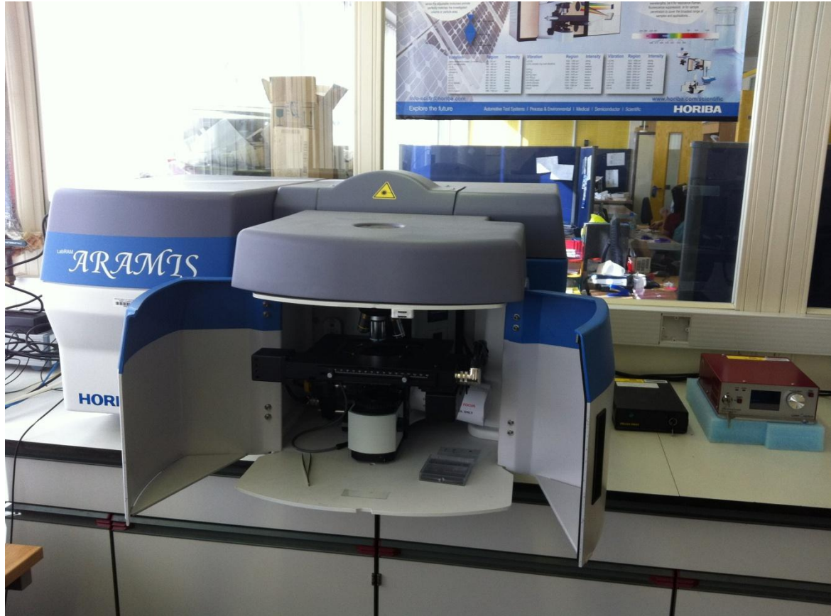
Figure 2.13. JY Horiba Labram Aramis imaging confocal Raman microscope used in this thesis, located in the Begbroke science park, Department of Materials, University of Oxford.
