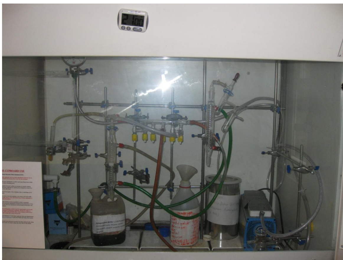
Figure 3.1. The schlenk line set up to synthesis Mn doped ZnSe quantum dots, located in 12/13 parks road, department of materials, University of Oxford.
