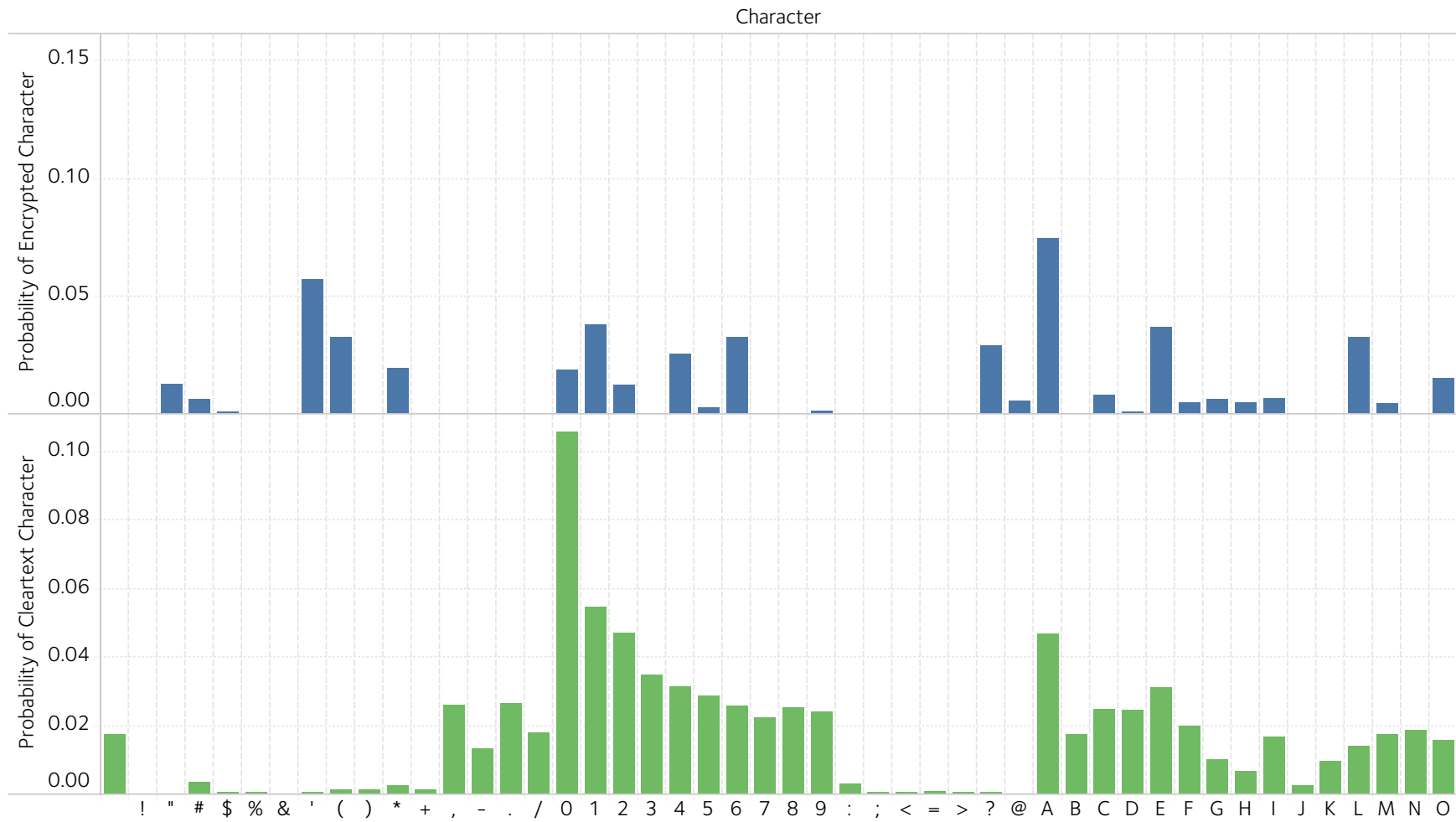
Figure C.1: Frequency analysis for key 01 over first half of the character set. Probability of each character in encrypted messages (top, blue) is compared against probability of the same character appearing in a cleartext message, calculated across all messages (bottom, green).
