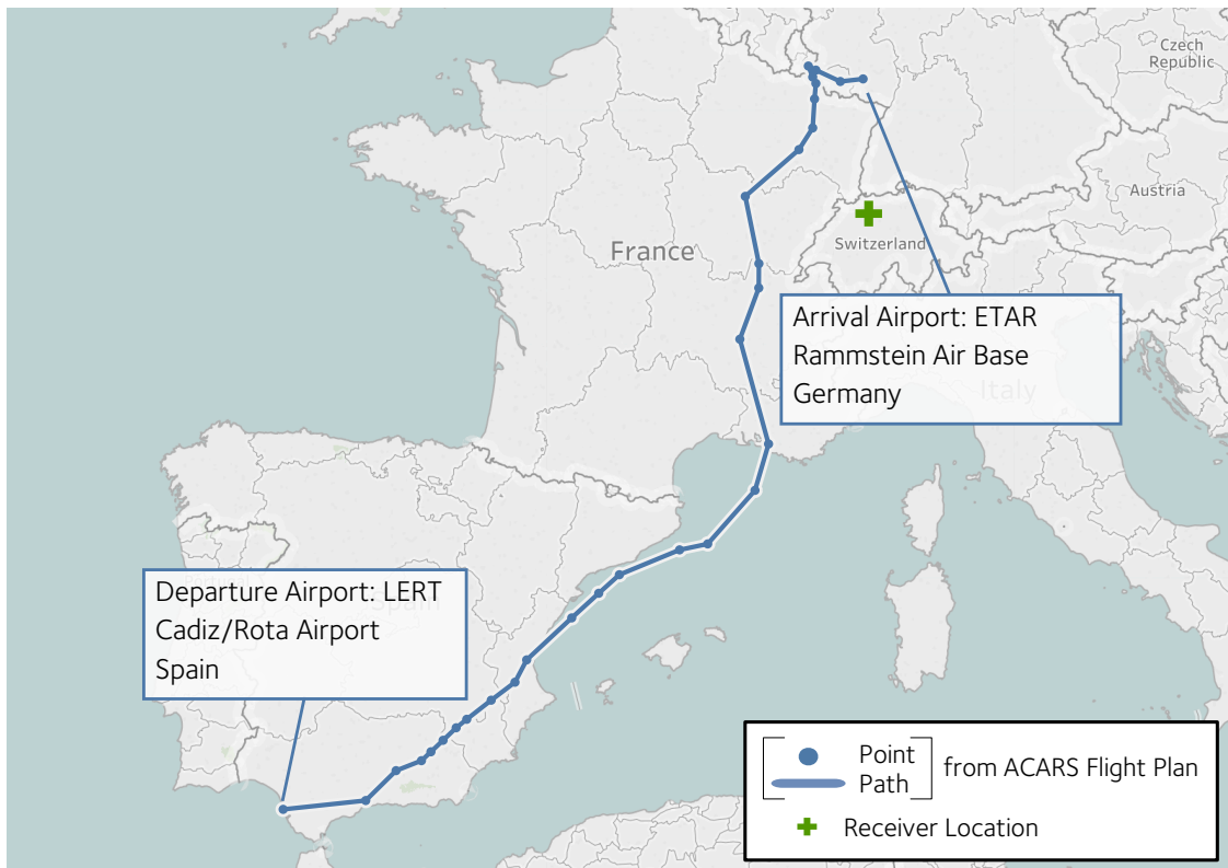
Figure 6.6: Plotted flight update from a US military aircraft in January 2017. This was collected on the SATCOM link.
