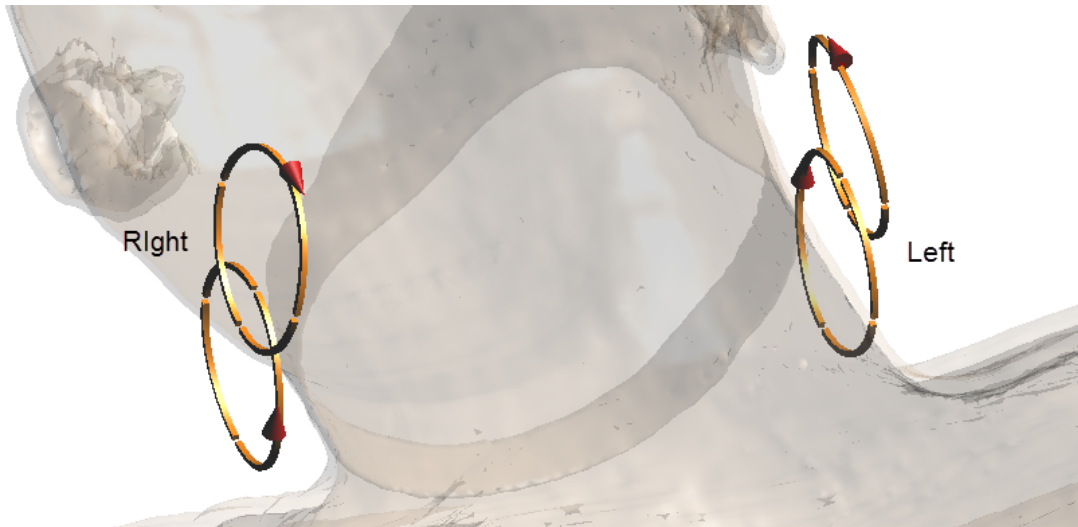
Figure 4.24: Illustration of the proposed receive array. Two loops of 50 mm diameter are positioned at each side, overlapping for decoupling.
