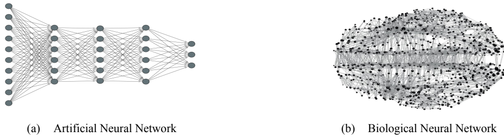
Figure 5.1: Difference in topology between an artificial neural network (left), and a sketch of a network of structural connections that link distinct neural elements in a brain (right) [62].
