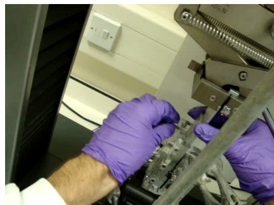
(f) Fastening lower gripper to Perspex box
