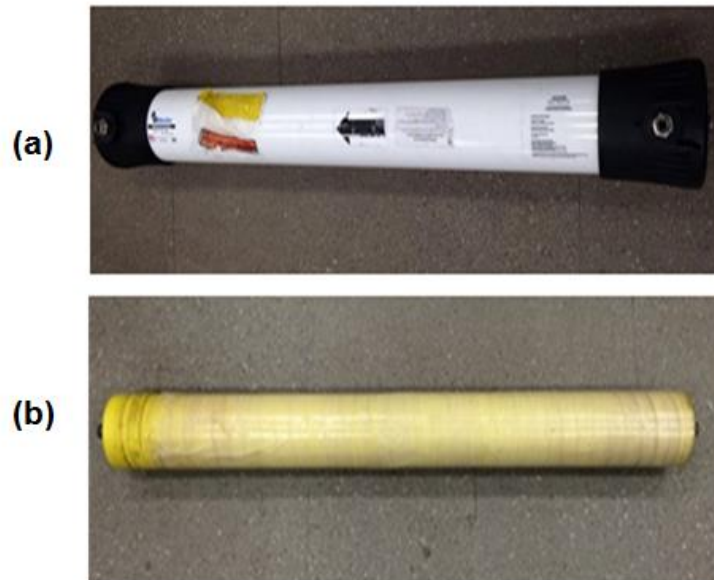
Figure 6.2: Spiral wound CTA membrane element (a) inside the module (b) out of the module
