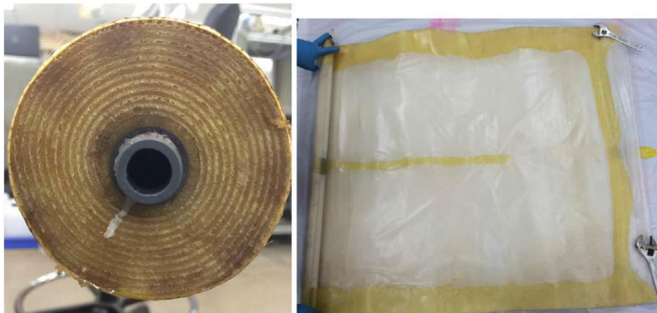
Figure 6.3: Cross-sectional view of the spiral wound CTA membrane taken out of its module casing (left) and unrolled (right).
