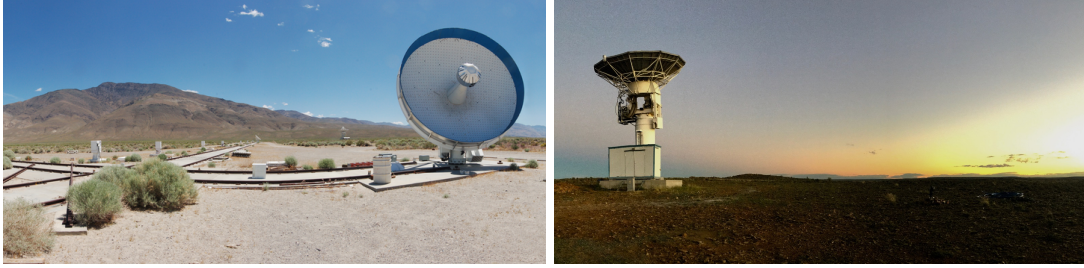
Figure 1 – (Left) The 6.1-m C-BASS North telescope at Owens Valley Radio Observatory. (Right) The 7.6-m C-BASS South telescope at Klerfontein, South Africa. Note that the horizon at C-BASS South is much flatter, which is expected to lead to less scan-synchronous groundspill. The overlap in sky-coverage between the two telescopes, and the different characteristics of their ground spillover signals, will allow us to partly break the degeneracy between ground emissions and sky modes that are symmetric about the celestial poles.
