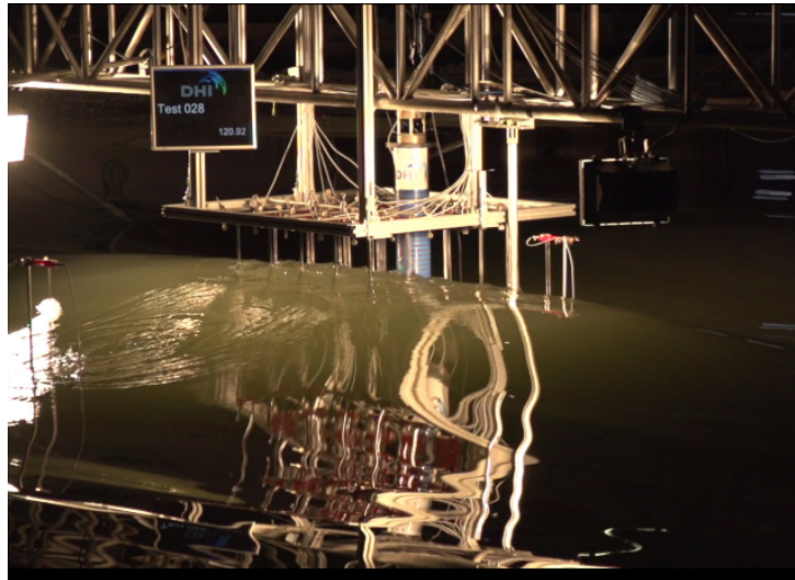
Figure 5.1: High speed photograph from DeRisk wave basin testing showing model monopile and wave (Bredmose et al. , 2016)
