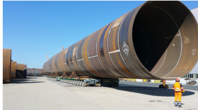
Figure 1.5: Fabricated monopile for Veja Mate offshore wind farm ( D = 7.8 m) (Windindustrie in Deutschland, 2016)
