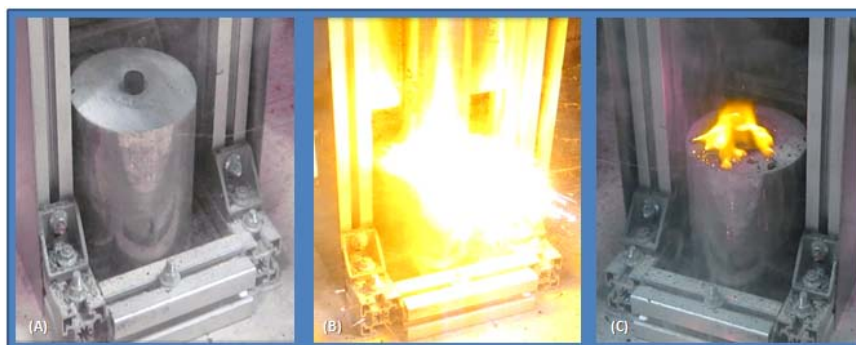
Figure 3: A 4-gram NaAlH 4 wafer ignited upon first impact (free fall height = 1 m)
