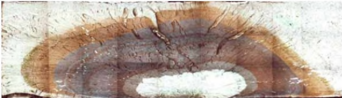
Figure 7 [58], showing subsequent steps of DHC, in a complete through-wall crack.
