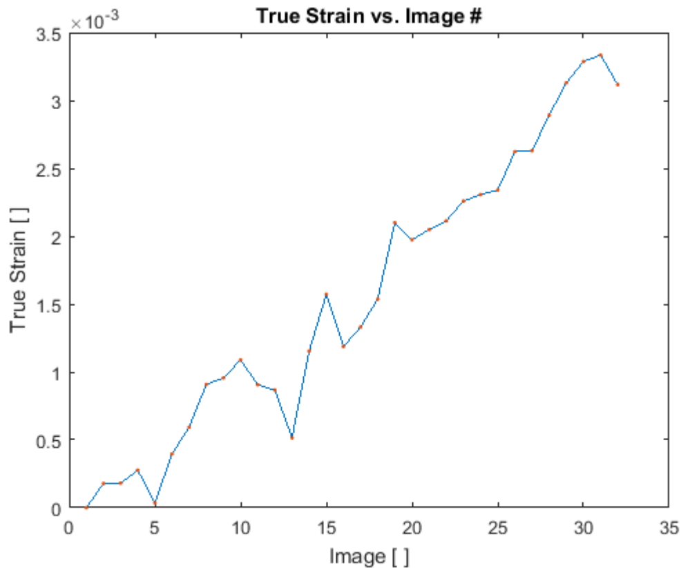
Figure 47 A strain graph calculated from the correlation shown in the previous figure. This is raw data without the removal of badly tracked markers. The positive strain shows an expansion of distance between markers. The final strain of 3.5 \times 10^{-3} is reached progressively as the trench is deepened and more stress is relieved.
