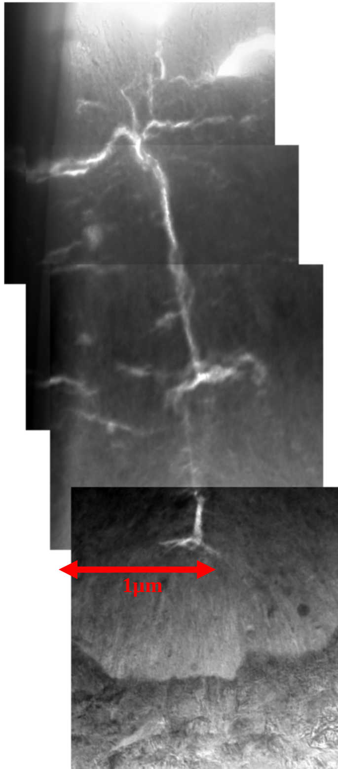
Figure 34 Composite TEM micrograph of the double transition sample liftout. This image clearly shows the vertical crack, which extends from the exterior of the oxide to the edge of the oxide formed during the secondary exposure. The metal substrate shows features that indicate the build-up of dislocations as suggested by Tejlund [84].
