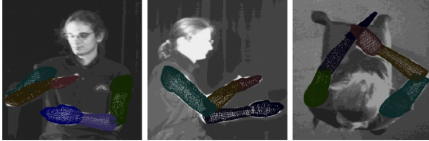
Figure 2.8: Multi-camera system of Vogler and Metaxas (1998) to segment out the hands and arms in 3D.
