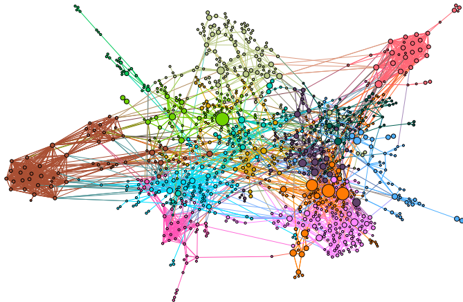
Figure 5.3: Hyperlink network of Wikipedia pages of the considered mathematical concepts (see [206]). The size of the nodes is proportional to their PageRank [34] (calculated with standard parameters) and the color coding corresponds to communities found using the Louvain algorithm [24].
