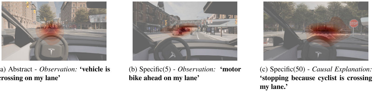
Fig. 4. Sample screenshots and the generated explanations (including observations announcement and causal explanations) from the three driving scenarios. Heatmaps of gaze points from all the participants are plotted over the images, indicating areas of interest. In the Abstract scenario (Fig. 4a), all movable/dynamic non-human actors are referred to as ‘Vehicle’. Thus, a cyclist was referred to as a vehicle. Fig. 4b depicts a scene from the Specific(5) scenario in which the AV’s perception system accurately identified and classified a motorbike and provided a fine-grained explanation for this. In the Specific(50) scene (Fig. 4c), the AV’s perception system misclassified a pedestrian as a cyclist. The fine-grained/specific explanation provided exposed this error.
