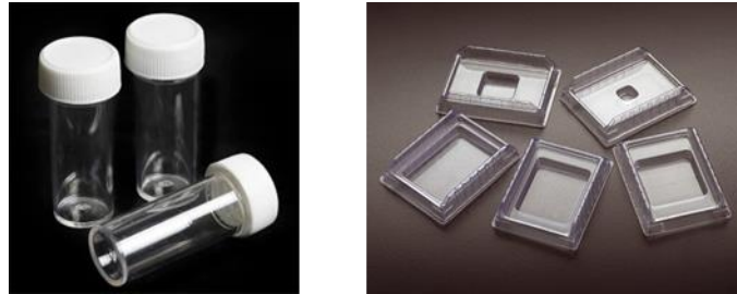
Figure 13: 7ml Bijou tubes were used for sample collection and fixation before embedding in OCT in histology moulds.
