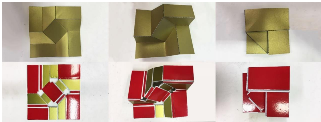
Figure 3.13 Folding sequence of a square-twist pattern with thick panels based on the offset crease technique and its zero-thickness source pattern.
