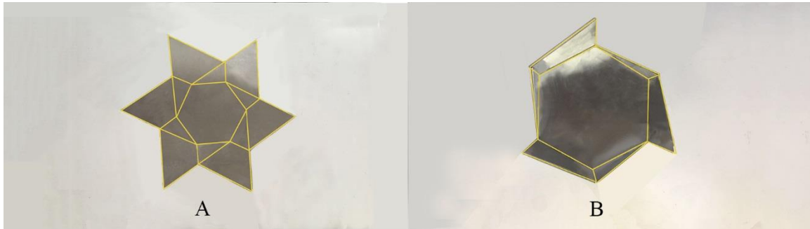
Figure 4.5 A rigid physical model for the winding membrane pattern in (A) the fully flat state and (B) the fully stowed state.
