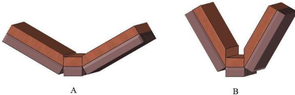
Figure 3.10 Adopting the offset crease method to alternative dihedral angles: (A) 120^\circ and (B) 60^\circ
