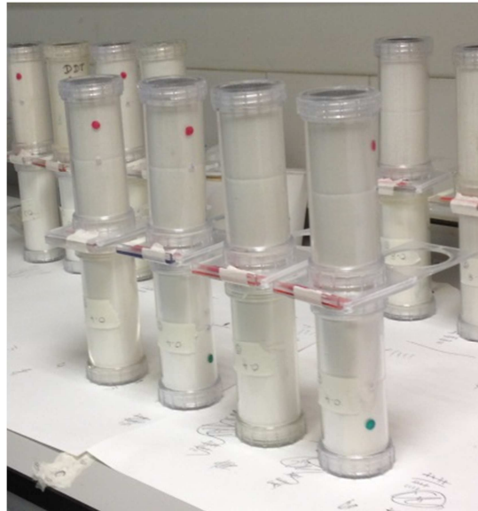
Figure 60: WHO insecticide resistance bioassay tubes. Top tube (red dot) is the test chamber, lower tube (green dot) is the rest chamber, separated by a plastic slider to either open or close the tubes to each other. The ends are secured by mesh, held in place by a plastic cap.
