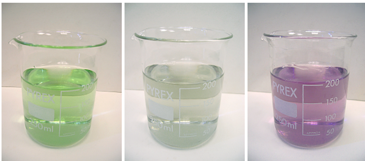
Figure 2.31: Colour change of the methyl-orange indigo-carmine indicator during a titration; from left to right : before, at, and after end point.
