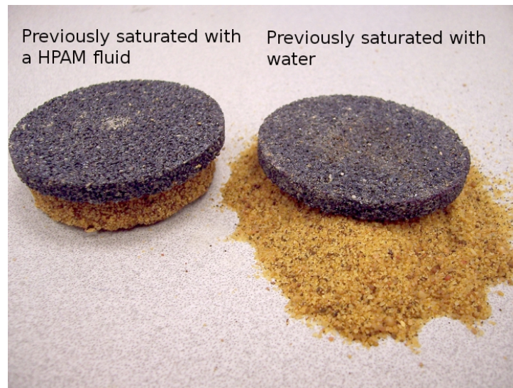
Figure 5.1: Strengthening effect of HPAM on dry Leighton Buzzard sand.
