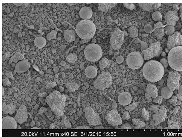
Figure 2.20: SEM micrograph of the blended additive 'EnhancIT 100'.
