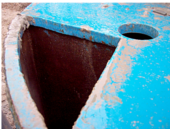
Figure 4.20: Digging bucket vent.
