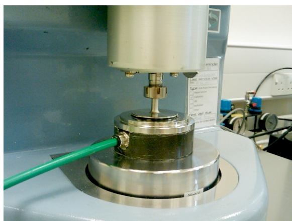
Figure 3.9: Measuring element of the rheometer in contact with a polymer fluid sample.
