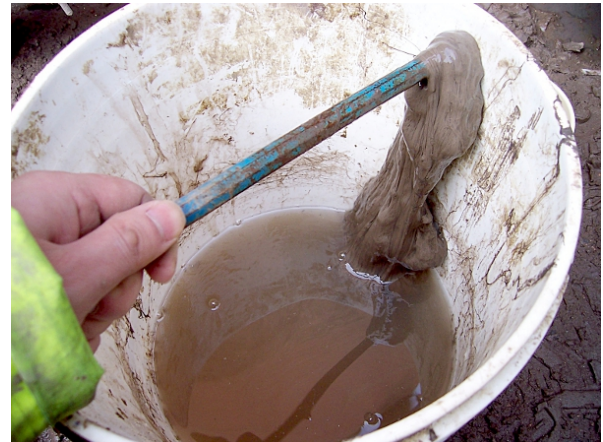
Figure 4.15: Effect of additive SlurryPro MPA on ‘dirty’ polymer fluids: left ) before addition; right ) after addition and stirring. (Photographs taken at a site in Glasgow, Scotland.)
