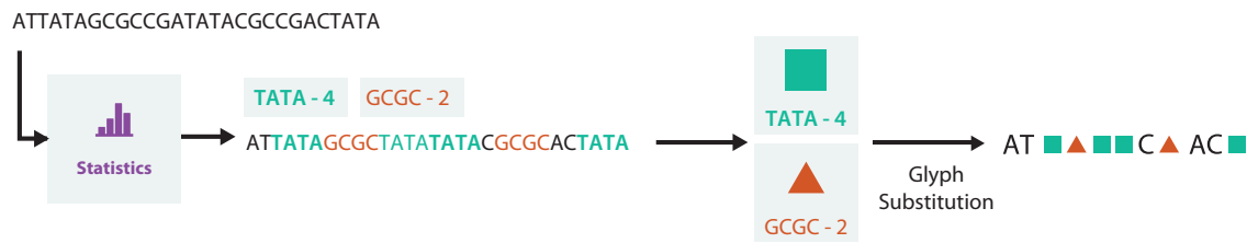
Figure 3.6: Text-based compression can use glyphs to replace common text with visual representations. In this case, some common DNA motifs are replaced with coloured shapes. Since reading text is a cognitively demanding process, showing structures of interest visually can speed up interpretation.
