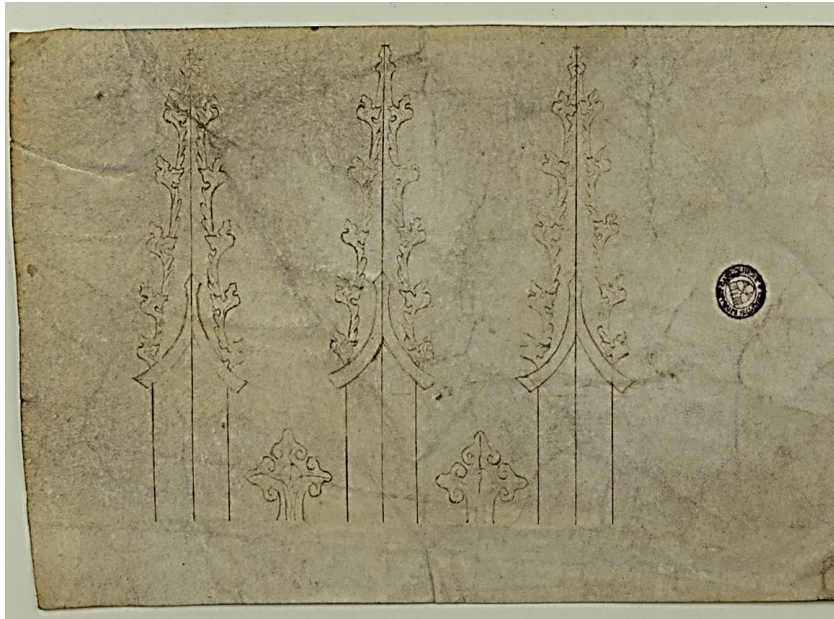
Fig 8.38 Canterbury Cathedral, possible design drawing for pinnacles of Central Tower for presentation to John Morton, attributed to John Wastell , c.1494 (CDC Chch Let 1_62)
