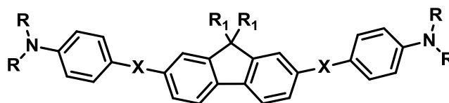
Figure 18: The donor-acceptor-donor fluorene platform. Aniline-based donors are connected to the fluorene acceptor core via a conjugated link.
