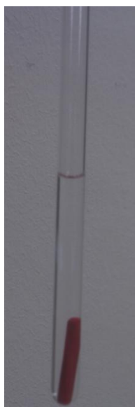
Figure 76: A magnetic stirrer bar (red) in D 2 O (0.5 mL) in an NMR tube. By placing the photolysis chamber on a magnetic stirrer, a satisfactory vortex could be created in the solution.
