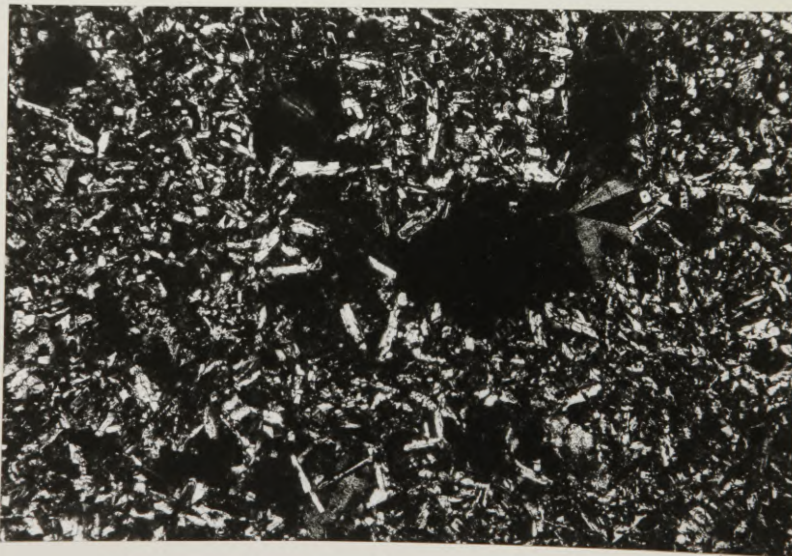
PLATE 24B. Same view as 24A but under crossed nicols. The presence of arrow-head twinning indicates that the silica polymorph on the right of the photograph is actually tridymite. Magnification x15.
