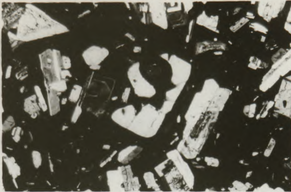
PLATE 18A. Photomicrograph of hornblende-hypersthene andesite (18640) from Chance's Dome. Slightly rounded, embayed and fractured quartz crystal and oscillatorily zoned crystals of plagioclase in a fine-grained to glassy matrix. Crossed nicols. Magnification x 18.9
