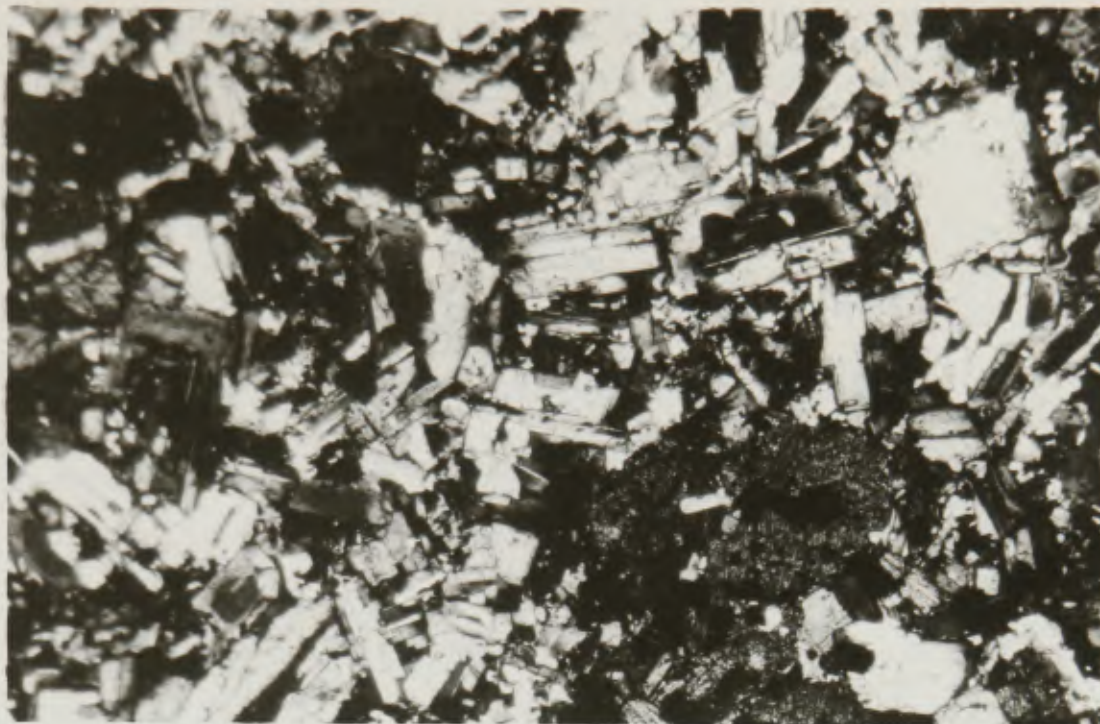
PLATE 26A. Photomicrograph of doleritic block (18597) from the White River Pyroclast Fall Series. The rock consists mainly of plagioclase with minor pyroxene and ore. The plagioclase which has cores of about An_{80} and rims of about An_{40} shows zoning predominantly of normal discontinuous type but slight oscillatory zoning also occurs. Crossed nicols. Magnification x 18.9.
