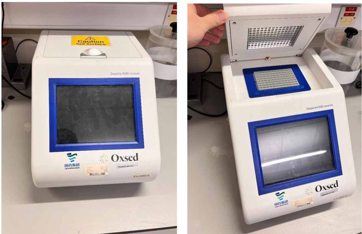
Figure 6.1 Sinopharm Colorimetric Reader. The Sinopharm thermostatic photometer is used to track real-time colour changes in LAMP reactions. This model was custom-built for Oxsed Limited [230] to facilitate high-throughput diagnostics, capturing images every 20 seconds for
