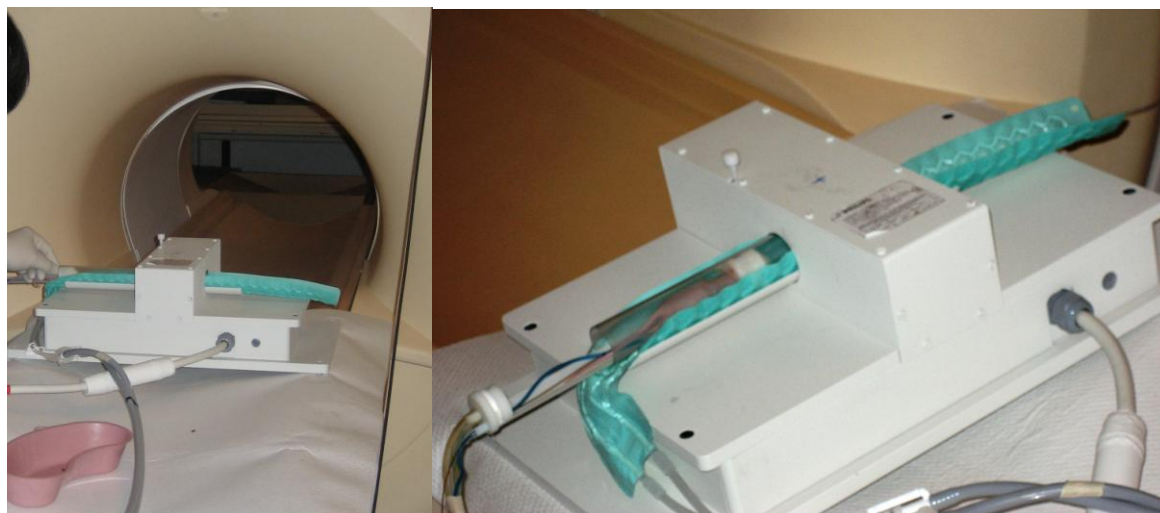
Figure 5-57: Solenoidal coil (inner diameter = 40 mm, coil length = 40 mm) used for single animal MRI. The animal was positioned in the center of the coil. The holding tube had continuous oxygen and anesthesia flow and was kept warm with a heating pad.
