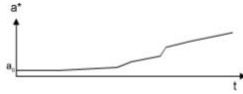
Figure 2.12 Design crack size history
