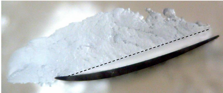
Fig. 15 Accretion at test end for the 10% melt ratio case. The original contact surface between accretion and aerofoil before rotation is shown by the black dashed line.
