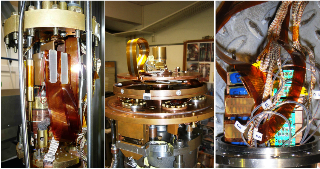
Figure 3.8: Photographs showing etched metal foil cabling after installation: (left) two 12-track-pair cables installed for readout of 5 SQUID sensors mounted in an Oxford Instruments K400 dilution refrigerator; (centre) a shielded cable installed for readout of NTD-Ge sensors within the EDELWEISS test cryostat at IPNL; (right) several 4-track-pair cables installed alongside their woven counterparts for readout of SQUID sensors at the CryoEDM experiment, Grenoble.
