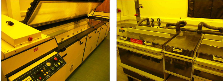
Figure 3.1: Equipment at the Oxford Physics Photofabrication Unit: ( left ) UV exposure unit; ( right ) etching bath.
