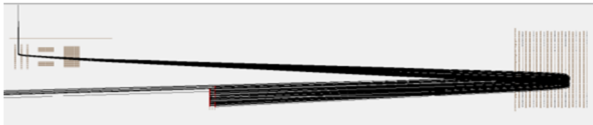
Figure 6.13: SIMION workbenches used to simulate the ion optics arrangement within the ToF mass spectrometer. a) The extraction optics, reflectron and MCP potential arrays (PAs) arranged in the same way as the components in panel d) of Figure 6.9. b) Au + ion packet containing 100 ions, with kinetic energies equally spaced in the range 29.5-30.49 eV, passing through the PAs, and landing on the offset MCP.
