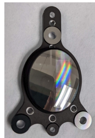
Figure 4. (left) Grating efficiency based on shaped groove modeling, wavelength dependent diffraction efficiencies, \rho_{g,\lambda_i} , where g is the order, are used in the instrument model. (right) Image of shaped-groove grating.
