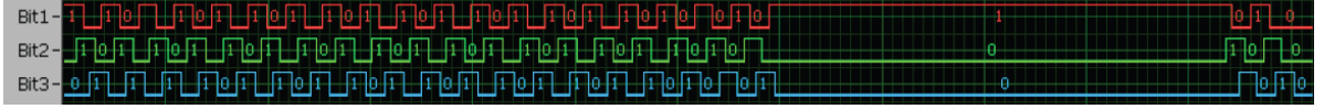
Figure 3.35: Sequence of the CCD clocks that pauses at the 19th CCD register.
