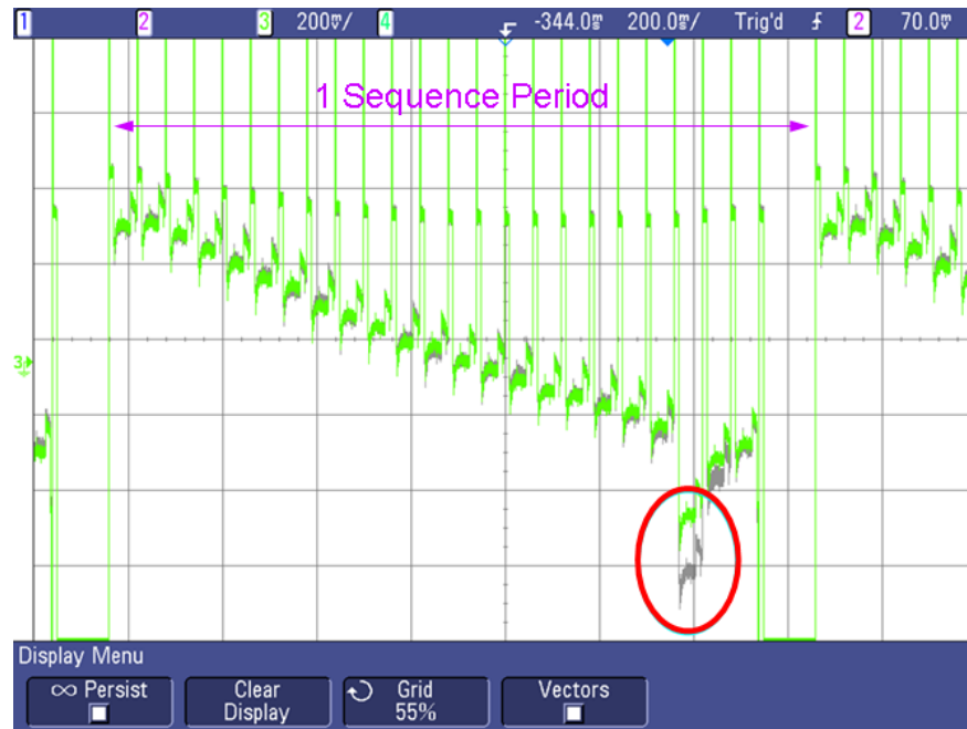
Figure 3.26: Oscilloscope trace of a successful charge transfer in the ISIS2 main array.
