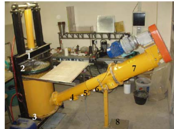
Figure 2.32. Experimental apparatus developed by Vinai (2006): 1) displacement wire Transducer, 2) top EPC, 3) bottom EPC, 4) pressure cell 1, 5) pressure cell 2, 6) pressure cell 3, 7) torque meter, 8) weighting platform (scale).
