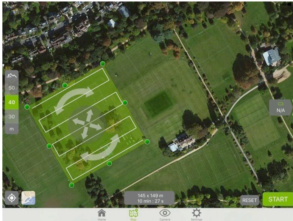
Figure 3.4 An example of the flight plan section of the Pix4D software (University Parks, Oxford, UK). The user can designate the area covered (light green square), and by using this information as well as the image overlap set by the user, the software determines the number of rows that must be flown by the drone over the designated area (in this case seven rows are indicated). The measured area is displayed as well as time of flight plan (grey box, centre bottom). The area covered here is 145 m x 149 m and will take approximately 10 minutes and 27 seconds. The altitude can be set using the slider on the left side of the screen, and is set to 40 m in this example.
