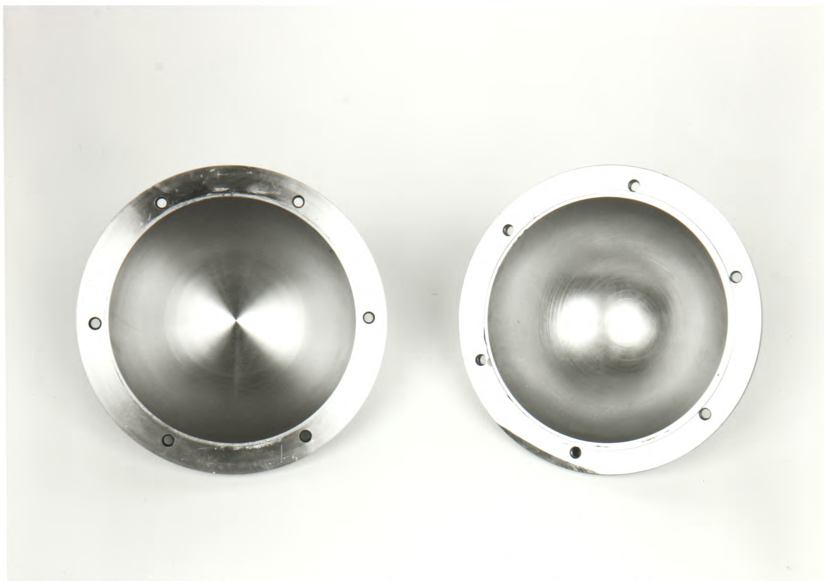
Fig. 4.2 Photograph of the two halves of the spherical mould used to cast wax into a spherical shape.
