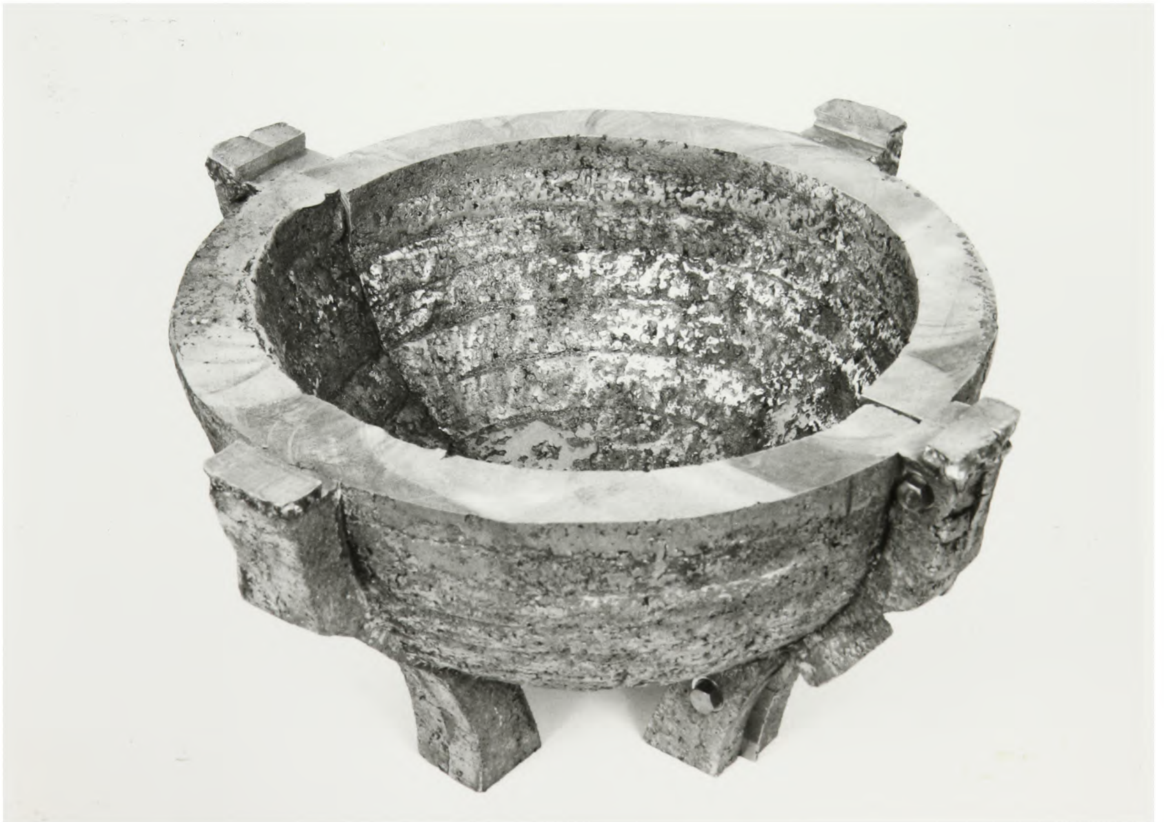
Fig. 7.3 Photographs of the cast aluminium male (above) with dural location plate attached, and both halves of the female (below) mould.
