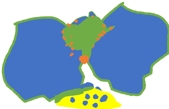
c) further diamond graphitisation along gap between diamonds, P < B-S line T > T_{\text{eutectic point of WC-Co}}
