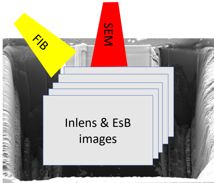
Figure 3.9: the configuration of FIB-SEM 3D tomography.
