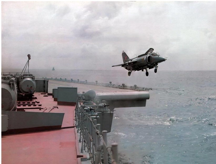
Fig. 6 – Kiev-class aircraft-carrying ship launching Yak-38 Forger vertical take-off and landing fighter. Note SS-N-12 Sandbox anti-ship missile canisters on the left of the picture. (Public domain).
