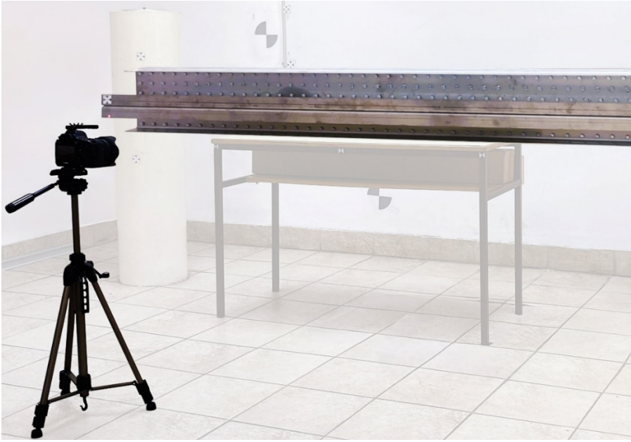
Fig. 4 The photogrammetric method used for measurement of specimen imperfections.
